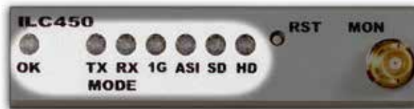
Figure 6. ILC450 Front Panel Status LEDs
