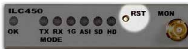
Figure 8. ILC450 Reset Switch
